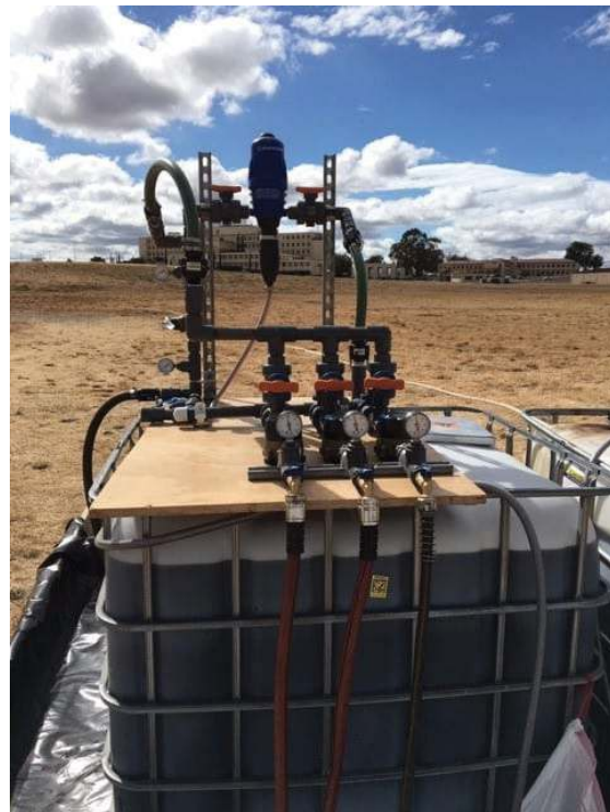
TRAVIS AIR FORCE BASE’S SUSTAINABLE GROUND-WATER TREATMENT PROGRAM (GWTP) USING SOY OIL ACCOMPLISHED THE DUAL GOAL OF COST SAVINGS AND ENVIRONMENTAL PROTECTION.
