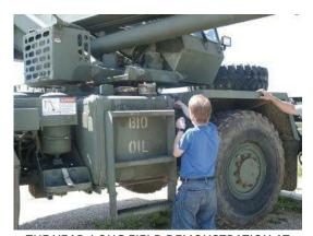
THE YEAR-LONG FIELD DEMONSTRATION AT FORT LEONARD WOOD, MO., FOUND THAT ALL FIVE OF THE BIOBASED HYDRAULIC FLUIDS THEY TESTED PERFORMED WELL IN ALL OF THE EQUIPMENT.
